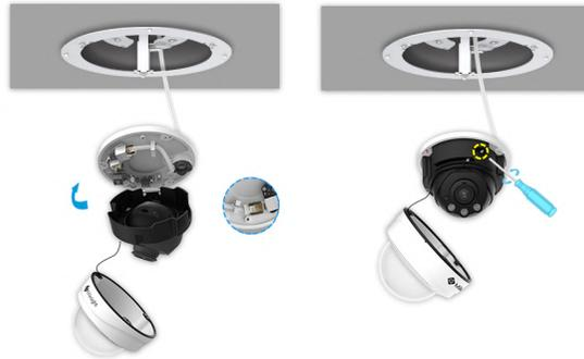
**Step 10:** Rotate the camera anticlockwise to the mounting bracket and make sure it is positioned correctly. Then lock the camera with the mounting adaptor by tightening the loosened set screw on Step 3;
