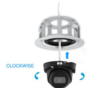
**Step 5:** Tighten the loosened set screw in Step 2 to lock the camera with the mounting adaptor;
