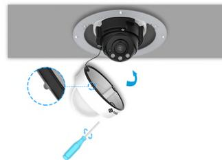
**Step 13:** Put the magnetic ring cover on to complete the installation.
