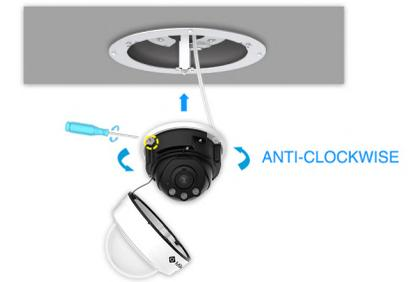
**Step 11:** Loosen the clamp screw on the camera, adjust the lens to the correct direction and tighten the clamp screw;
