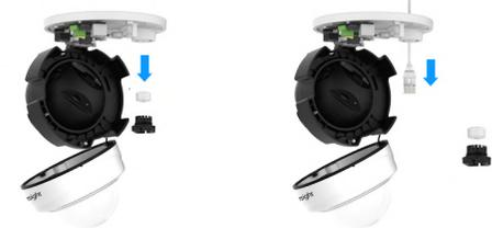
**Step 8:** Place the piercing cap on the cable and then push the cable through the waterproof flange grommet. Pull the flange grommet with the cable into the entry hole and make sure it is securely seated in the inside and outside of the cable entry hole;
