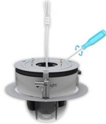
**Step 6:** 2.Connect the cables and insert the camera with mounting adaptor into the drilled hole;
