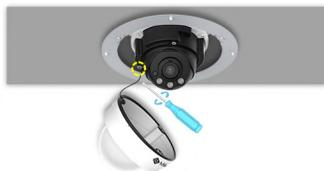
**Step 12:** Attach the dome cover by tightening 3 loosened screws on Step 3 and make sure that the groove on the dome cover is aligned to the one on the camera;
