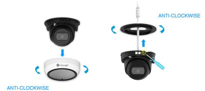
**Step 4:** Rotate the camera to the mounting bracket and make sure it is positioned correctly;
